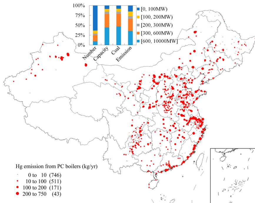
**Figure 4.** Geographical distribution of Mercury emissions from PC boilers (the size of the circle represents the annual mercury emission and the numbers inside the parentheses are the quantities).
