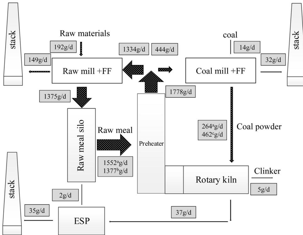
**Fig. 1.** Mercury mass flows in Plant 1.
