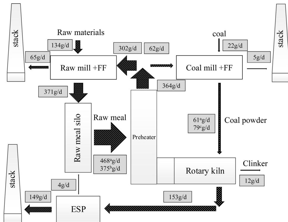
**Fig. 2.** Mercury mass flows in Plant 2.
