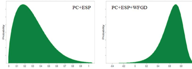
Figure 2. Probabilistic distribution profile of mercury removal efficiency.
