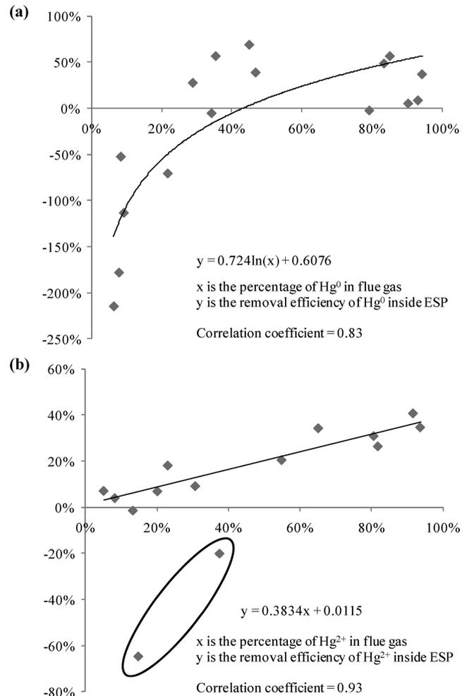
Figure 3. Relationship (a) between the percentage of  $Hg^0$  in flue gas and the removal efficiency of  $Hg^0$  inside ESP; and (b) between the percentage of  $Hg^{2+}$  in flue gas and the removal efficiency of  $Hg^{2+}$  inside ESP.
